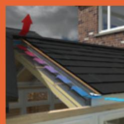
With many unproven roof conversions, moisture can form inside the roof causing staining and mould growth to the internal plasterboard, leading to deterioration or even failure of the roof components.
